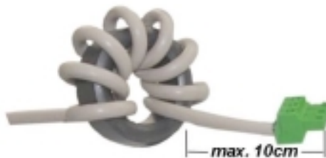
Figure 11: RS232 Interface Line on a Ring Core
